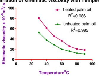
Variation of kinematic viscosity with Temperature
